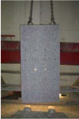
Test of light behind typical concrete panel for Future gallery concrete panels walls. Photo: Jennifer Turner.
