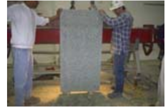
Prototypical concrete panel with rebar holes. Photo: Jennifer Turner.
